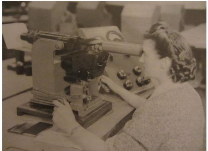
Two production lines and testing of a gun sight for span calibration, fore and aft drift and gyro magnetic centre at the Ashington Factory.
